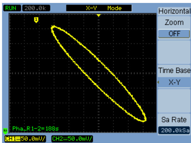
Figure 15 X-Y Display Format Showing Out-of-Phase Waveforms
